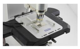
The PE120 heating and freezing stage
