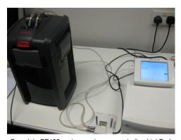
Complete PE120 system— stage, controller, LinkPad and ECP water pump in the Lab
