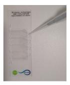
In just one step, push the piston down till the first resistance to load the loading area. The chamber will be filled by capillarity. If chamber is loaded in more than one step air-bubbles could be inserted inside the chamber. Thus, affecting the reliability of results.
